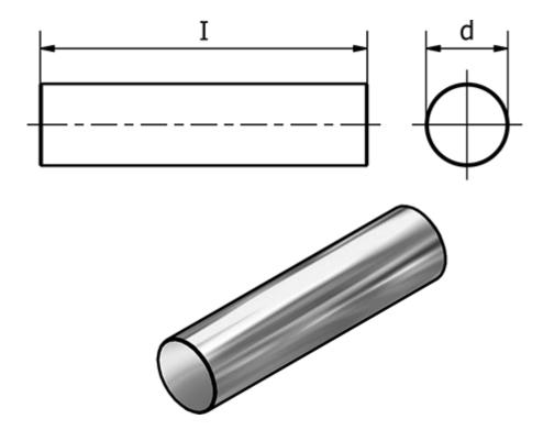
$\begin{array}{ll} \text{d1} & = 3 \\ \text{I} & = 12 \\ \text{Nominal adhesive forces} = 1.3 \\ \text{Weight in g} & = 450 \end{array}$
